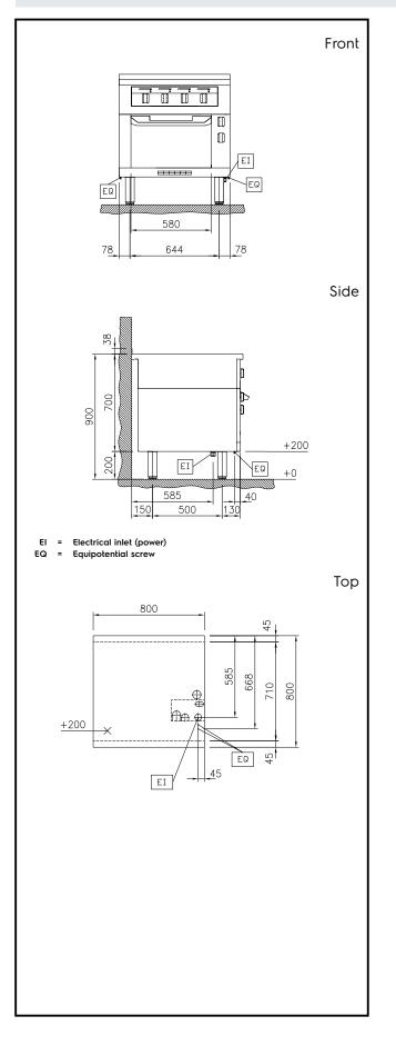
Modular Cooking Range Line thermaline 80 - 4 Zone Induction Top on Oven, 1 Side with Backsplash H=700 The company reserves the right to make modifications to the products without prior notice. All information correct at time of printing.
